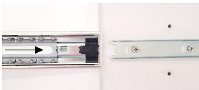
A) Ensure the ball bearings are slid forward before reconnecting.
