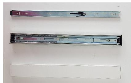
Turn the slides over & extend them fully until you can see the black disconnect lever. Pinch it in the direction of the arrow. This will release the slide members.
